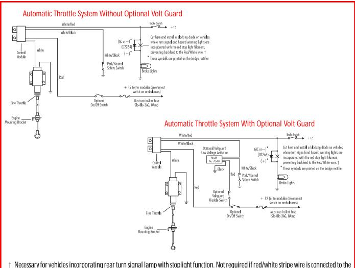
† Necessary for vehicles incorporating rear turn signal lamp with stoplight function. Not required if red/white stripe wire is connected to the Center High Mount Stop Light (CHMSL) circuit. May substitute Radio Shack #276-1185 or Westinghouse #MB12A25V05.
