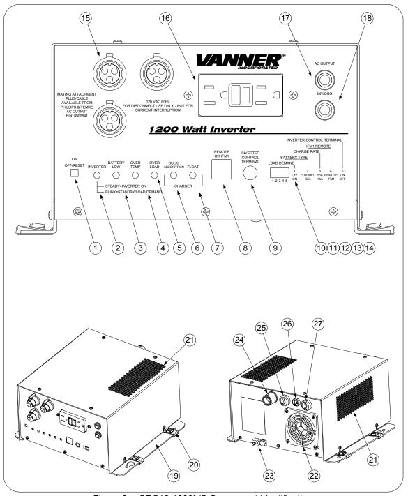
Figure 2 SRC12-1200L/S Component Identification
