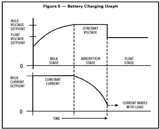
Figure 1 Battery Charging Graph
