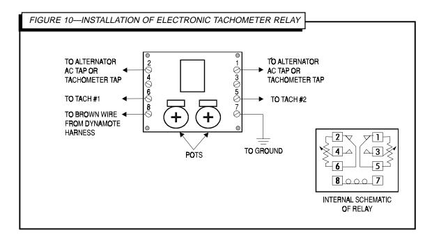
Electronic tachometer relay calibration procedure:
