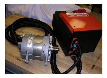
Figure 1. A 4kW Dynamic inverter system for a work truck
