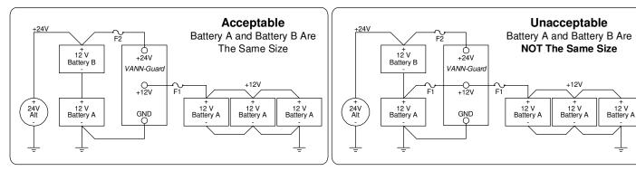
In certain applications, such as private coach or alternate energy applications, it may be desirable to have additional 12 volt "House Batteries" to operate heavy 12 volt (inverter) loads. Use the *VANN-Guard* to charge the additional batteries.
